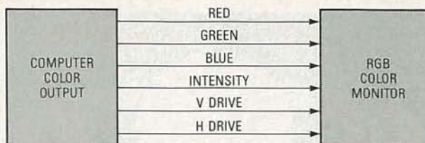
FIG. 3—AN RGB COLOR SIGNAL is also non-NTSC and TTL. Each of the three primary colors is provided as a separate signal along with the intensity and vertical and horizontal drive signals. Like the TTL monochrome monitor, the RGB monitor integrates the separate signals into a complete color display.
