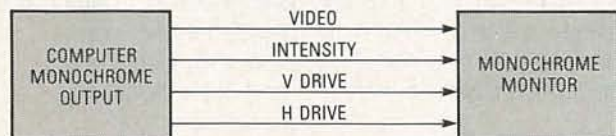
FIG. 2—A COMPUTER WITH an IBM-type monochrome output provides individual TTL signals (non-NTSC) for the video component, intensity, and the vertical and horizontal drive. The monitor integrates the four signals into a screen display.
