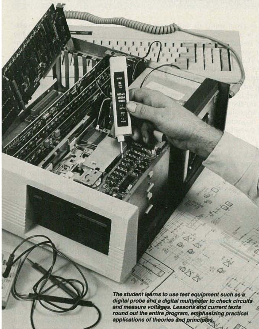
Installing the disk-drive in the PC is one of the final stages in the assembly of the microcomputer. Learning the use of test equipment to check circuits is an integral part of the training which, with field experience, develops invaluable career skills.
